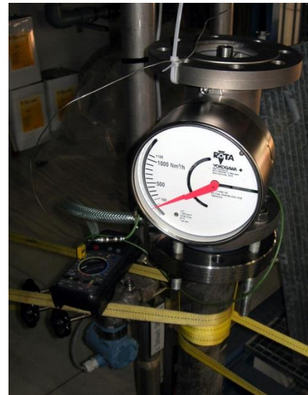
Fig. 9 Comparative tests with the flow sensor FIC4-10
