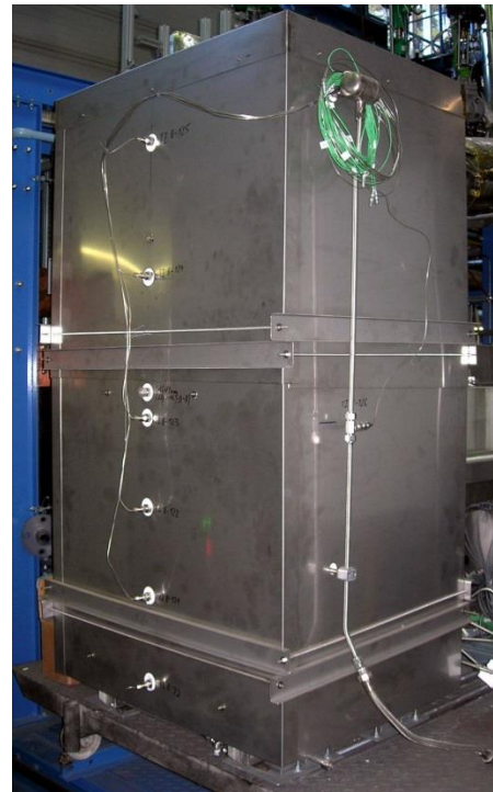
Fig. 4 RPV simulator, insulated with Multitherm
